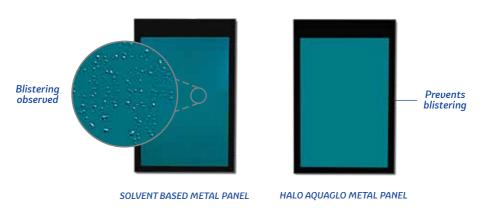
GLOSS TEST Panels under accelerated heat and light exposure for 250 hours in standard testers in our lab
